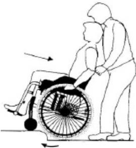
Drive the wheelchair backwards as close as possible to the edge of the threshold. Drive down from the threshold very slowly and pull back the wheelchair on the rear wheels until the front casters are free from the edge. Then lower them onto the base.
