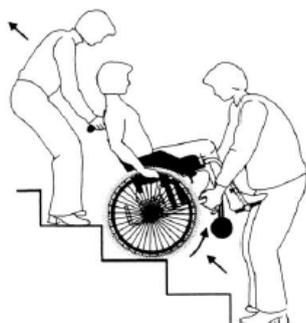
Push the wheelchair to the stair touching the first step with the rear wheels. Use the handles to incline the wheelchair backwards. The second Attendant should grasp the lower front corners of the frame. Carry the wheelchair by the backrest barrier, never by the folding handles - these can be damaged.
