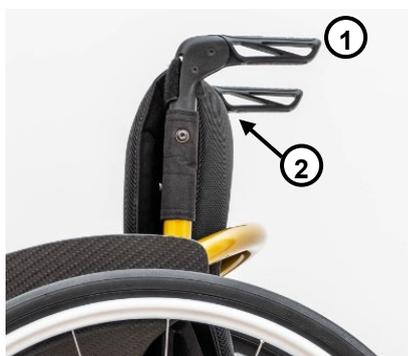
The method of unfolding the push handle:
