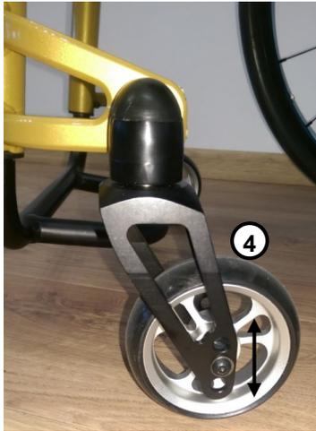
To change the seat height, you can mount the front wheels in different positions (4). (This picture uses a front fork with 3 different positions). Different holes also allow the installation of front wheels with different diameters.
