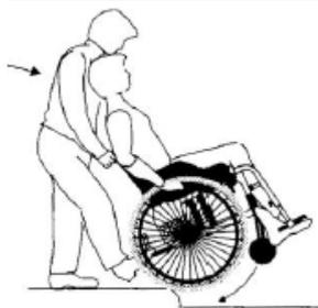
Incline the wheelchair backwards with use of the step pedal allowing the front casters to come off the base as much as it is necessary. Drive the wheelchair slowly from of the edge and carefully lower the front casters onto the base.
