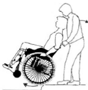
Drive to the threshold so that the rear wheels touch the edge. Tilt the wheelchair backwards with use of the step pedal allowing the front casters to come off the base as much as it is necessary. Pull the wheelchair backwards on the threshold until the front casters are above the threshold. Then carefully lower the front casters onto the base.
