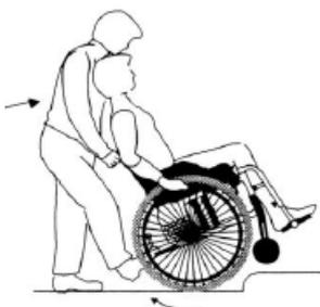
The Attendant inclines the wheelchair backwards by using the step pedal, allowing the front casters to come off the base. Drive forward until the rear wheels touch the edge. Use the handles at the back of the wheelchair to lift the rear wheels on the threshold.
