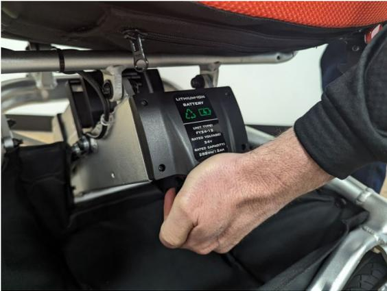
To remove the primary battery, pull the release lever up and slide the battery towards you.
