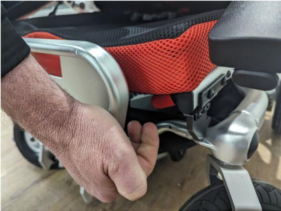
Pull the red release lever located under the seat cushion.
