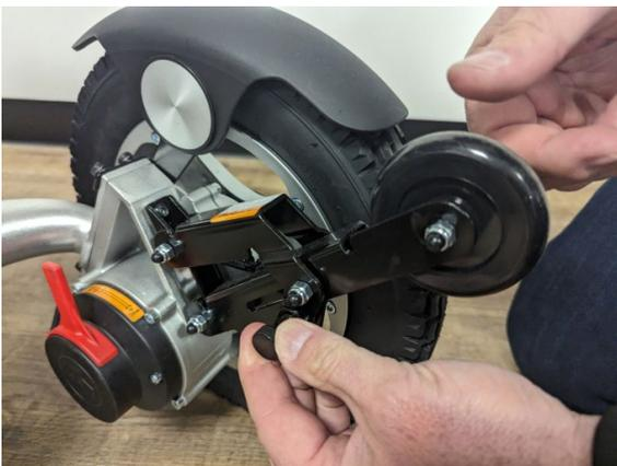
Fold the anti-top wheels in by pulling out the adjustment knob and pushing them up and towards the chair.
