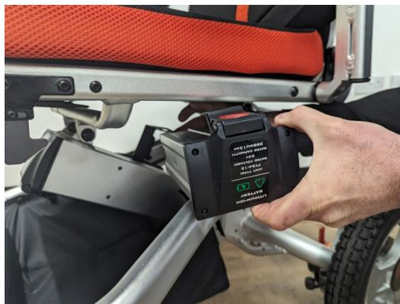
To remove the secondary battery, pull the release lever up and slide the battery towards the front of the chair and then rotate it outwards and pull towards you.
