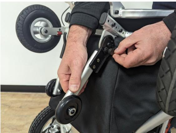
To open the climber wheels, pull the release knob out and lift each climber wheel up until it locks into position.
