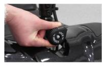
4. Lock the steering by pulling the locking knob out and turning 90°.
