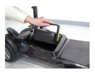
2. Pull up the battery handle and then lift the battery pack out of the battery compartment.
