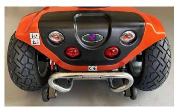
Up = Electromagnetic Brake is engaged (Drive Mode)
