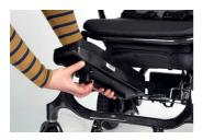
9. Install the seat cushion which attaches with velcro.
