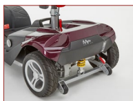
Rear monoshock suspension
