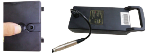
Photo 22. Conduct a deep discharge every month
