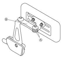
Remove upper screw and friction cap A.
