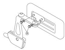
Loosen the two screws (A).
