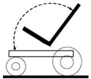
Fig. 3-5 Drive slowdown due to backrest angle
