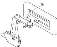
Remove hip pad bracket from mounting slot via cut-out  $\ensuremath{\mathbb{B}}$ .
