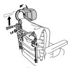
Loosen the handwheels  $\ensuremath{\mathfrak{A}}$  and raise the push handles as far as possible.
