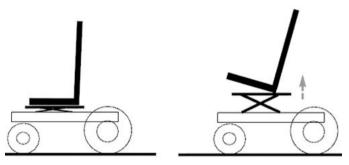
Fig. 3-4 Home position (left), drive slowdown due to height (right)
