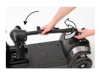
5. Turn the tiller knob anti-clockwise to loosen tiller. Lower the tiller and then turn the tiller knob clockwise to secure.
