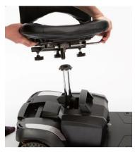
5. Replace the seat and rotate it until it locks in to its correct position.
