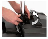
4. Lower battery pack in to the compartment in the scooter and then turn the handle to secure the pack in place.
