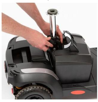
Place the battery pack in to the void in the scooter and ensure it sits flush. Press lightly on the top of the battery pack to ensure the battery pack is fully installed.
