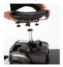
Push the Seat Rotate Lever whilst pulling up on the seat to remove.
