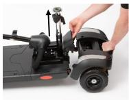
Pull up on the Connecting Handle to split the two halves of the base, whilst pushing on the rear of the scooter. 3. Loosen the tiller adjustment knob and pull up the tiller to the required height. Retighten the knob to secure.
