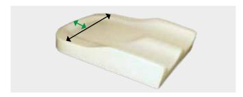
Rear cushion radius: +3.8 cm extra depth is designed to fill the gap between the seat and backrest/ upholstery. 1.25 cm decrease in total width allows cushion to fit both stated size and seats that are 2.5 cm narrower.
