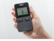
ECS remote control Indicates the health of the batteries and allows turning e-motion on and off from a seated position. Provides two assist levels and activates the roll-back delay.
