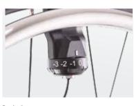
**Push-rim** Using the push-rim activates the motors for assistance. The sensitivity can be adjusted in just 7 steps.
