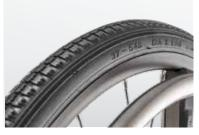
Tyre options Several tyre options are available (Rightrun 1\*, Marathon Plus 1\*, ProSpeed 1\* made of PU, Airless 1 3/8\* with PU-inlet)
