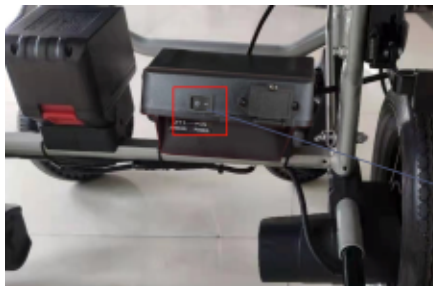
Main Power switch
