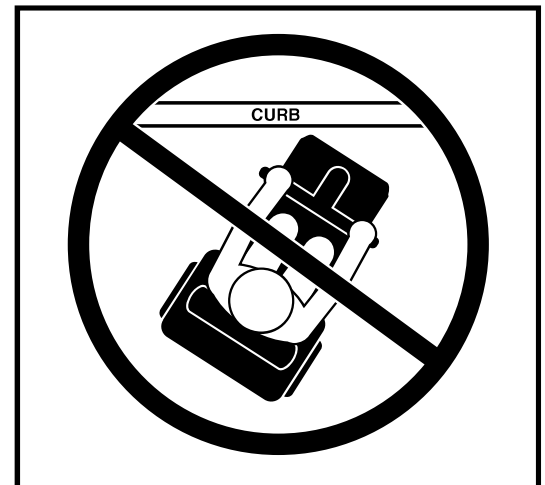
Figure 7. Incorrect Curb Approach
