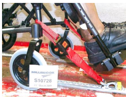
Fitting the front restraint
