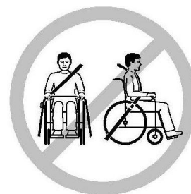
Incorrect seat belt position
