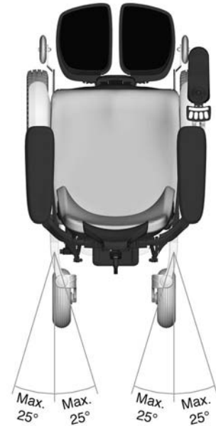
Figure 97. The angle of the loading straps must not exceed 25 degrees.
