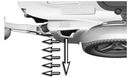
Figure 91. Releasing the brakes
