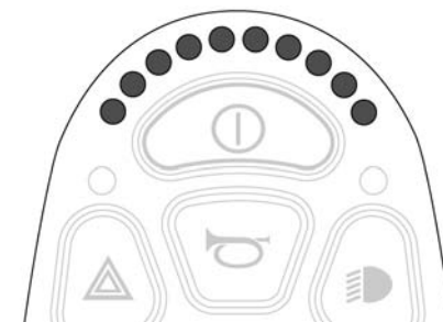
Figure 79. Battery Voltage Indicator
