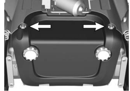
Figure 103. Knobs holding the front cover.
