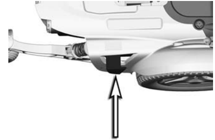
Figure 92. Resetting released brakes
