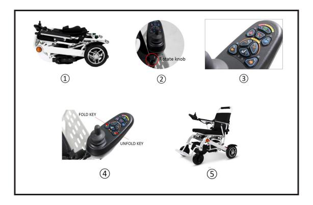
Your IGO Fold comes with automatic fold and unfold capabilities via a key fob as shown below.
