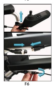
6. Mount the control panel and plug in the 5 –pin control cable in accordance with Fig. F6. (refer to the instructions on mounting the Control Panel)
