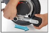
5. As shown in Fig. F5, press the anti-tipping wheel button and pull out the anti-tipping wheel.
