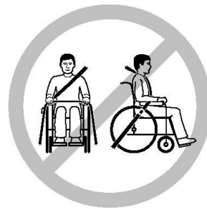
Incorrect seat belt position
