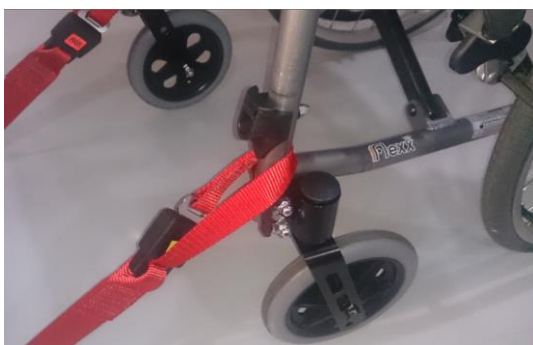
Fitting the Front Restraint
