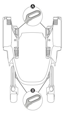
The wheelchair is equipped with four tie-down points used for transportation  $\blacksquare \checkmark \textcircled{B}$ . Two in the front O and two in the rear O.
