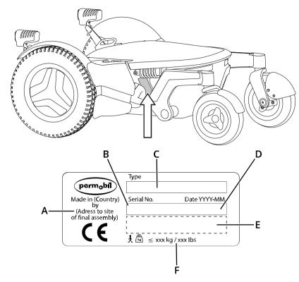
The serial number label is located on the lower, left-hand side of the wheelchair chassis. Look to the right of the drive wheel.
