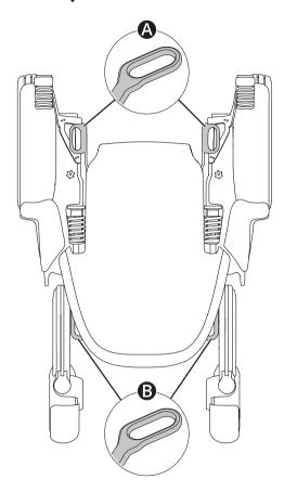
The wheelchair is equipped with four tie-down points used for transportation  $\rightleftharpoons$   $\overleftrightarrow{\bullet}$   $\boxdot$ . Two in the front  $\textcircled{\bullet}$  and two in the rear  $\textcircled{\bullet}$ .
