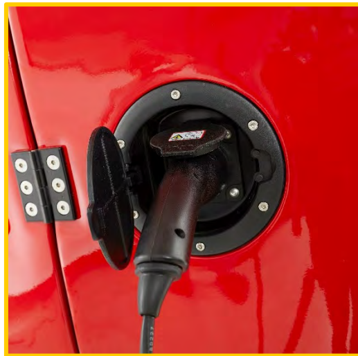
Figure 20 – External charge port open with external charge lead plugged in
