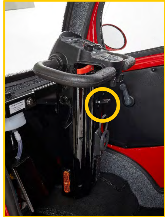
Figure 6 – Press the black handle down to adjust tiller pitch
