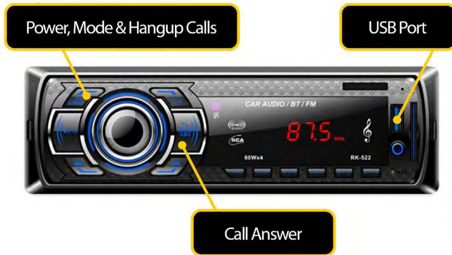
Figure 24 – Wireless Handsfree Control Unit (Key Buttons)
