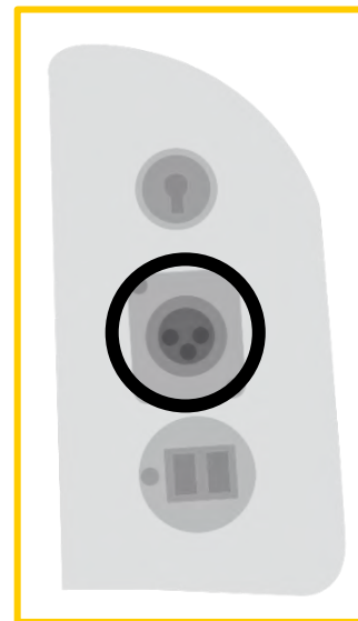
Figure 18 – Tiller mounted charge port
