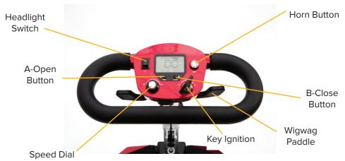
The scooter features an LCD display (right).
