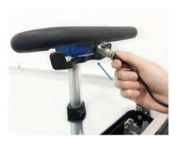
3. Insert the key into the ignition (as shown below) and switch the scooter on. Then press button on the tiller dash marked 'A-OPEN'. The scooter will then slowly beep and unfold. For safety, the unfold process will stop halfway. Press the button again to fully unfold the scooter. When fully unfolded the scooter will emit three quick beeps.
