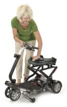
4. Finally push the tiller against the seat and the front of the floor pan towards the rear wheels to ensure your scooter is locked into the folded position.
