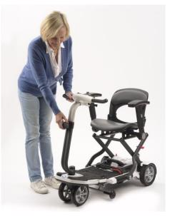
If you'd like to adjust the height of your tiller simply turn the adjustment wheel anti clockwise until the top part of the tiller moves freely up and down. Then just move the top half of the tiller to the height you would like and tighten the adjustment wheel by turning it clockwise until tight.
