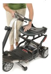
3. Use one hand to push the seat down towards the floor pan and the other to move the tiller towards the seat which will lift the front wheels off the floor and fold your scooter.
