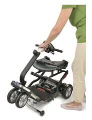
3. Ensure your scooter is locked in the unfolded position by pulling the seat away from the floor pan with one hand and pushing the tiller away from the seat with the other until you hear a click and feel you scooter lock into this position. Once your scooter is locked in position you will no longer be able to move the tiller towards and away from the seat so use this as a simple test to find out if you scooter is locked in the unfolded position.
