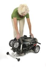
Once folded you can then lift your scooter using the handle at the rear and stand it on its front wheels to move around in the folded position.
