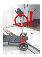
8. Pull the seat yellow push back, lift-up placement.
