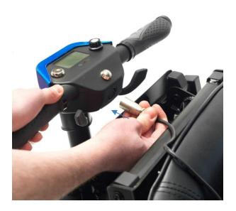
To charge your scooter, position the front of the unit next to a standard electrical outlet. Plug the charger into the scooter, and then into the electrical outlet. When the batteries are fully charged remove the charger from the scooter.
