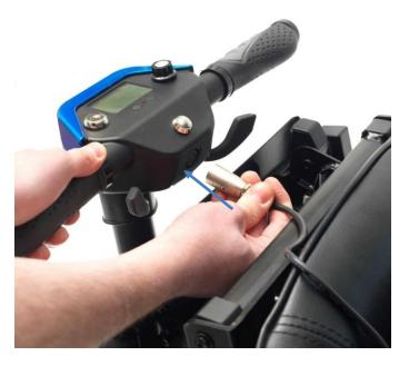
Insert the key in to the ignition (as shown below) and switch the scooter on. Then press the right hand side button (arrowed) for 1 second. The scooter will then slowly beep and unfold. For safety, the unfold process will stop halfway. Press the button again to fully unfold the scooter. When fully unfolded the scooter will emit three quick beeps.
