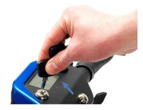
4. Insert the battery pack as shown below.
