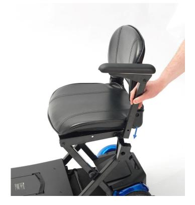
9. Secure the armrest by screwing in to the threaded knob in to the hole (arrowed).
