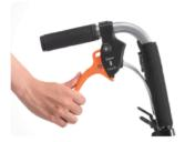
**P&P BRAKE** (Dual Function Braking System) The dual function braking system allows carers to slow or stop the wheelchair.
