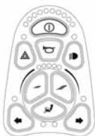
Control panel with lighting and seat functions.
