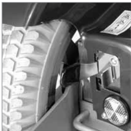
Released brakes with safety catch
