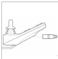
Charger connection point for the R-Net control panel
